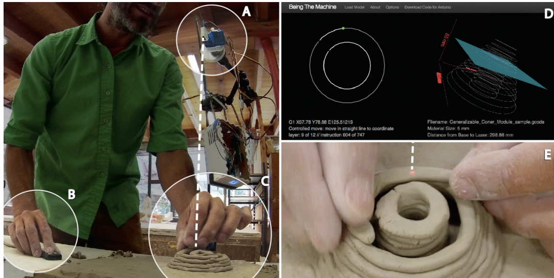
Figure 2.6: Being the Machine, machine-guided manual fabrication of 3D objects in which form is more emergent than predefined [6].
