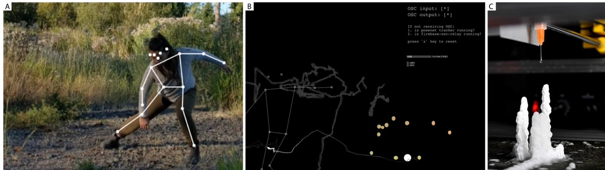
Figure 4.1: Re:Forming development occurred across remote settings using (A) a laptop camera to capture the dancer’s movement, (B) custom software to stream pose estimation data and translate the data to fabrication toolpaths using (C) a 2-axis CNC with the Liquid-Crystal Printing syringe for depositing and crystallizing sodium acetate trihydrate.
