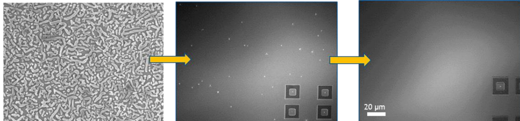
Figure 45. Representative SEM images of identical samples showing the improvement in selectivity with changing growth parameters.
