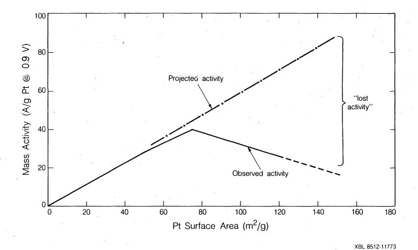
Figure 2. Activity - Pt surface area correlation observed with phosphoric acid fuel cell cathodes.
