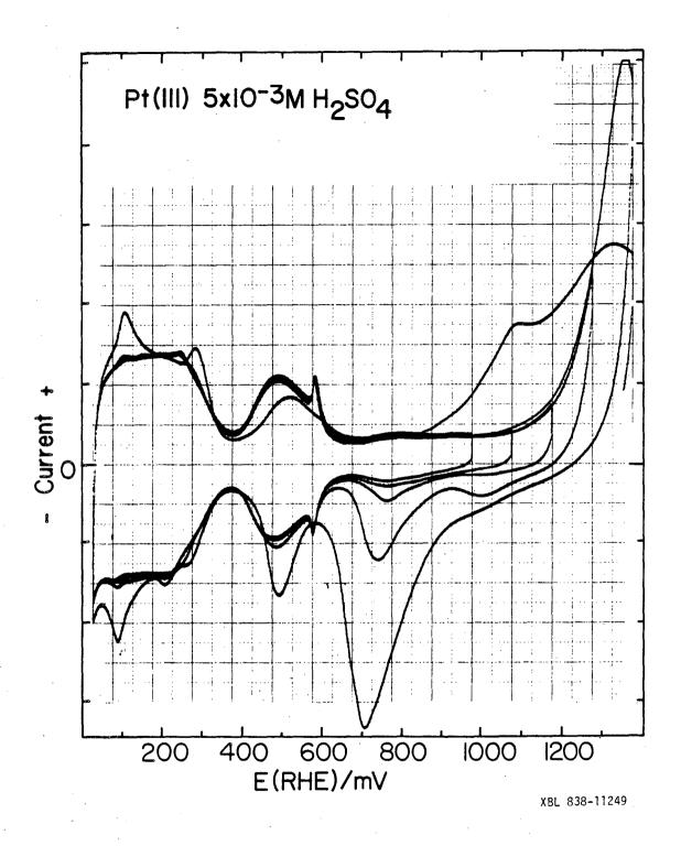
Figure 3. Voltammetry of UHV prepared Pt(111) surface.
