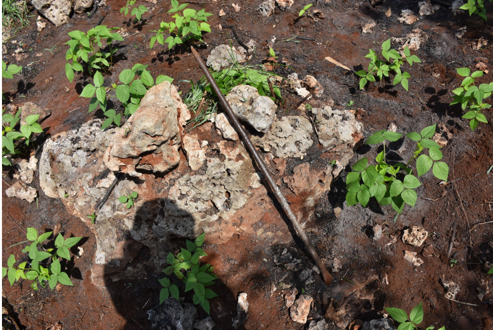
Figure 6-27. An mtaimbo , a long straight crowbar used to dig holes in the coral bedrock ( kupiga makongo ).
