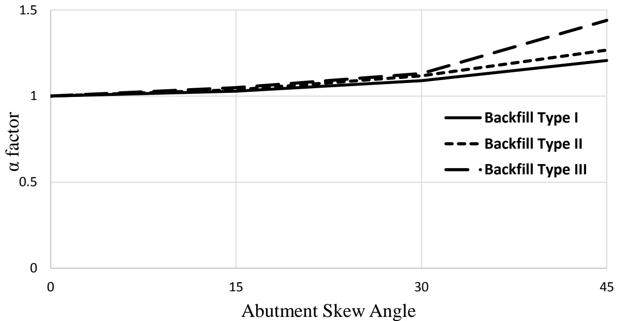
Figure 3-14: Comparison of \alpha factor in Bridge B with three representative GHFD backfill models (Soil Category I to III) and ductile shear key
