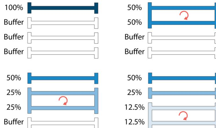
Fig. 4.1 **Dilution ladder topology** using ladder topology a sample can be 1:1 diluted and stored by connecting and mixing two subsequent steps of the ladder together
