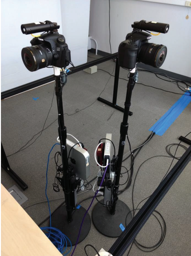
Figure 7. High-dynamic-range luminance mapping apparatus.
