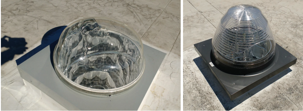
Figure 11. The two types of dome tested: clear ( left ) and prismatic ( right ).
