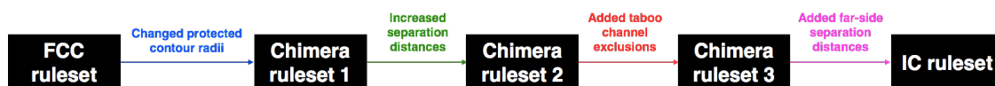
Figure 11.5: Block diagram showing how the chimera rulesets were created from the FCC and IC rulesets.
