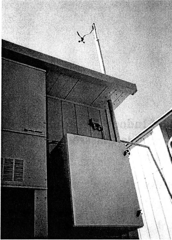
Figure 20: Photograph of the outdoor weather station to continuously measure local wind speed, wind direction, outdoor T and outdoor RH.
