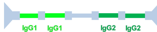
Fig. 7.2: Schematic of a four-node pore with two consecutive segments functionalized with IgG1 isotype-control antibody and two consecutive segments functionalized with IgG2 isotype-control antibody. The device dimensions were 25 \mu\text{m} x 25 \mu\text{m} (H x W) with five 1150 \mu\text{m} long segments separated by four nodes, each 65 \mu\text{m} x 50 \mu\text{m} (W x L).
