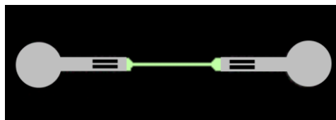
Fig. 3.6: Image showing the connection of the pore and reservoir layers. The green region indicates where the initial pore layer had been patterned. The reservoir mask is aligned such that the pore connects the two reservoirs of each device.
