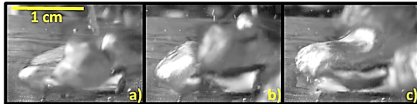
Fig. 4.8 At CHF ( q \approx 151 \text{ W/cm}^2 ) the isolated bubbles covering the heater as in Fig. 4.6p between large bubble ebullition cycles are replaced by a constant vapor film. These images are shown at 16ms intervals; image (c) shows the appearance of wave-like nodes at heater edges, and anti-nodes at the center at CHF.
