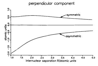
The kinetic energy contribution to the parallel and perpendicular components of the interaction nuclear magnetic shielding tensor of the  ${}^3\Sigma_u^+$  state of  $H_2$ , shown versus internuclear separation, as calculated using the electron gas theory of [2]. The curves labelled 'asymmetric' result from the use of  $T_0$ , while those labelled 'symmetric' result from the use of  $T_0'$ .
