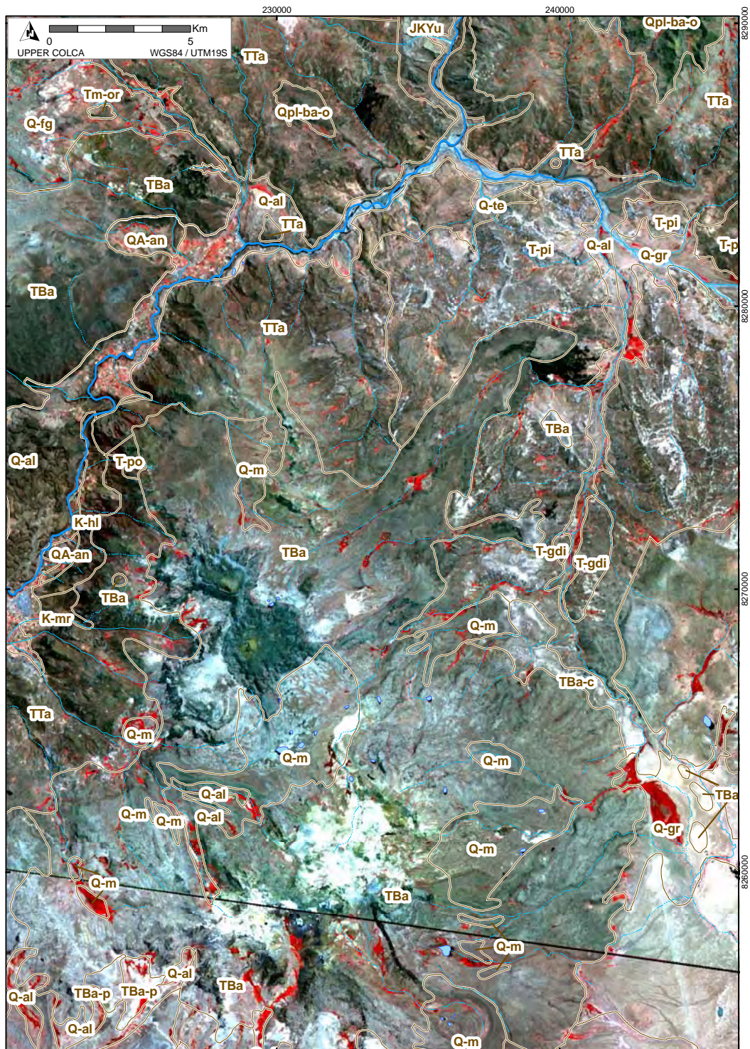
Figure 4-16. Geological map units shown on ASTER scene from 28 Sept 2000; legend is shown in Figure 4-14. In general, red pixels show areas of photosynthesizing vegetation (bofedales).
