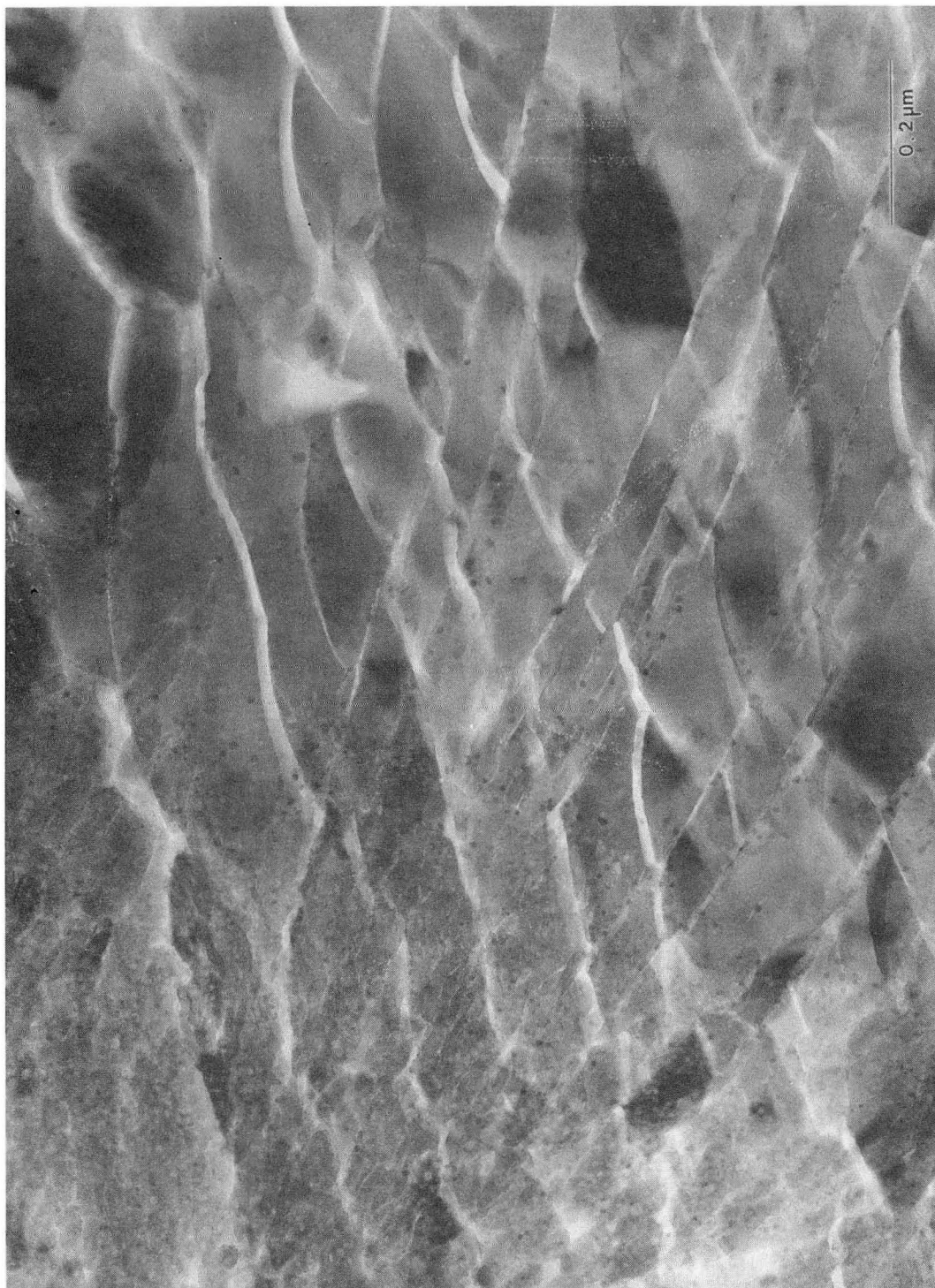
Figure 4.8 - Bright field TEM image of a thin section of a FeZSM-5 particle grown from an unstirred gel with \text{SiO}_2:\text{Fe}_2\text{O}_3 -ratio \simeq 200 , that has been steam treated at 700^\circ\text{C} for 4 hours. Note the inhomogeneous distribution of second phase particles throughout the FeZSM-5 particle. XBB 886-6204
