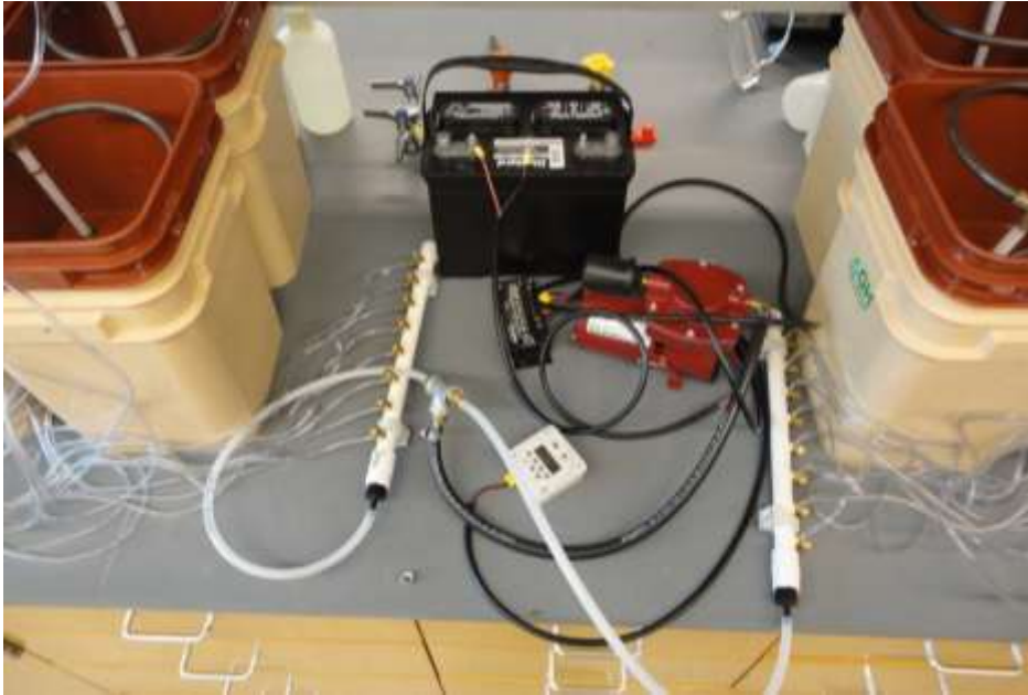
Riverside Pump System: battery, pump, timer, manifolds, air lift tubing
