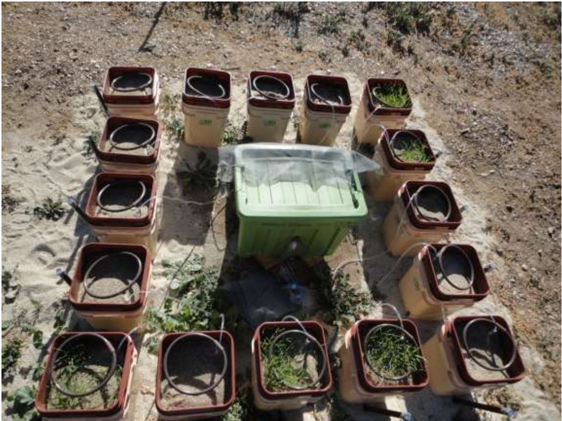
Figure 2.3. The ITNI modules deployed at Riverside, California. Modules with plants are invasive plant treatments and the other modules are controls. The green tote houses the air compressor and battery. Air distribution lines connect to the air-lift system in each module.
