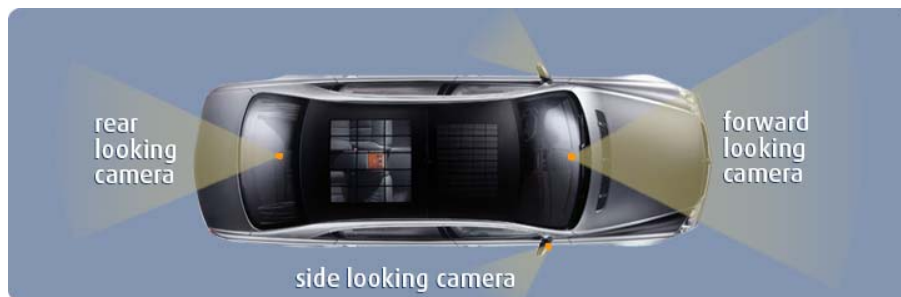
Figure 5-1 View angle of on-vehicle cameras
