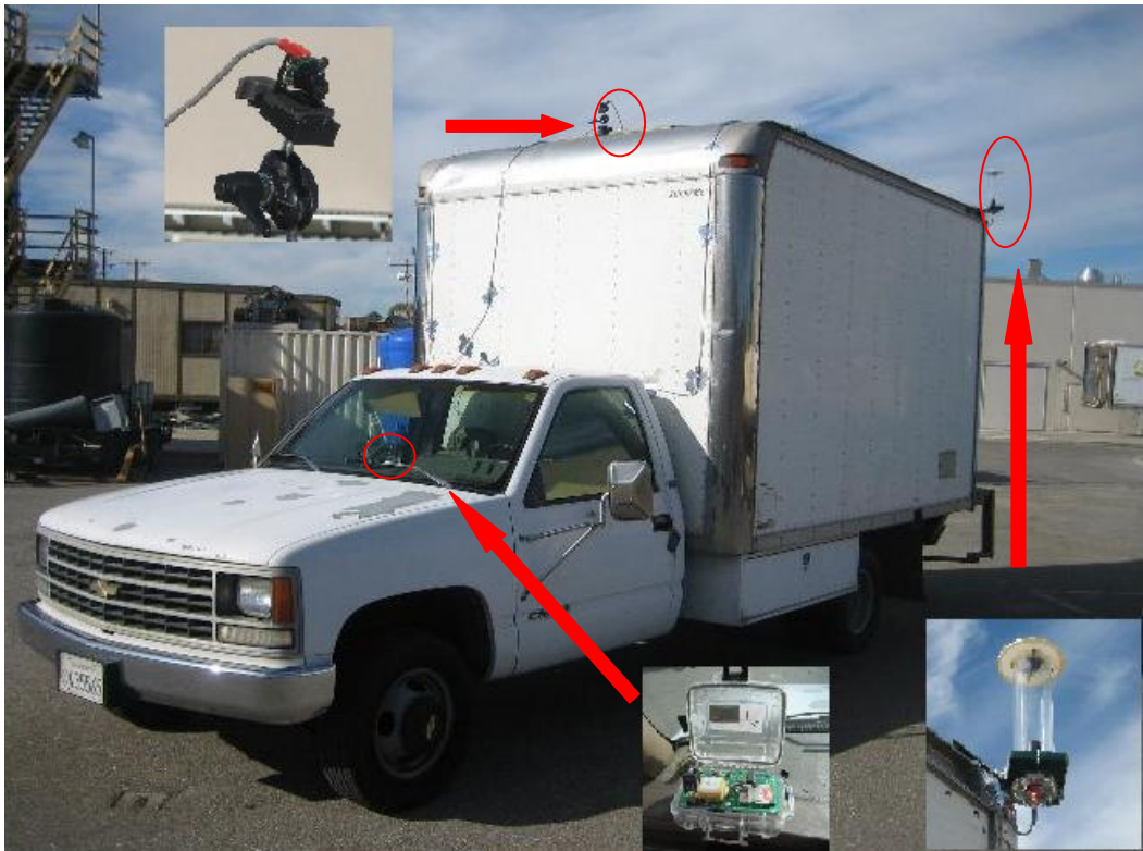
Figure 5-3 Vision sensor and GPS-equipped vehicle
