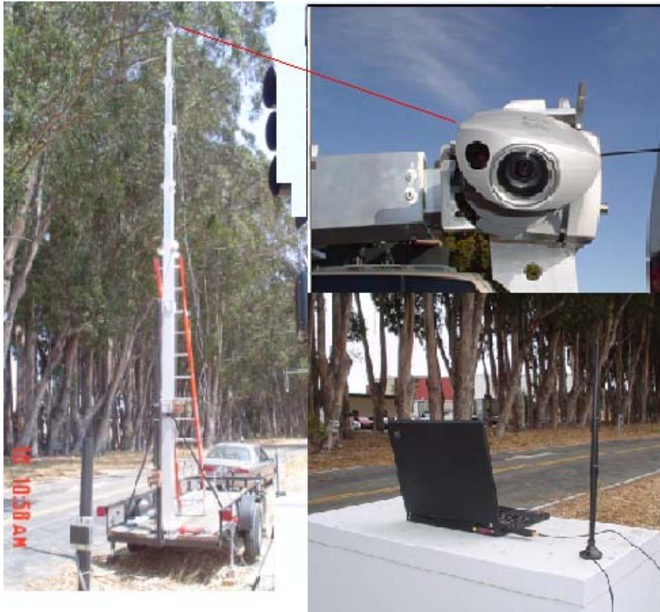
Figure 4-2 Mobile retractable pole setup
