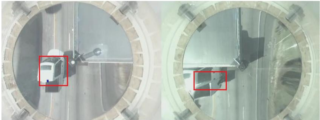
Figure 5-10 Duplicated detection in multiple sensors
