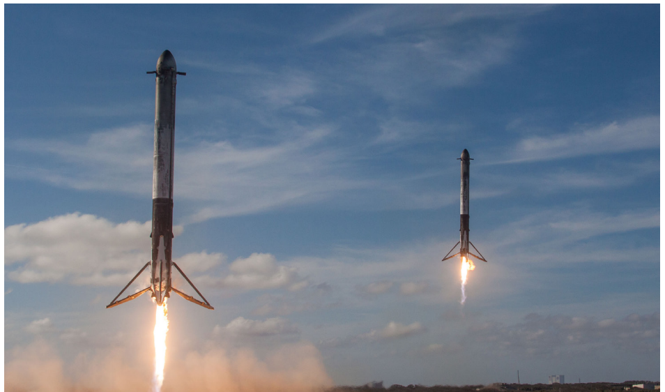
Figure 2. SpaceX is on the road to reusable rockets with their Falcon Heavy boosters, shown displaying the ability to land safely after a launch. 14
