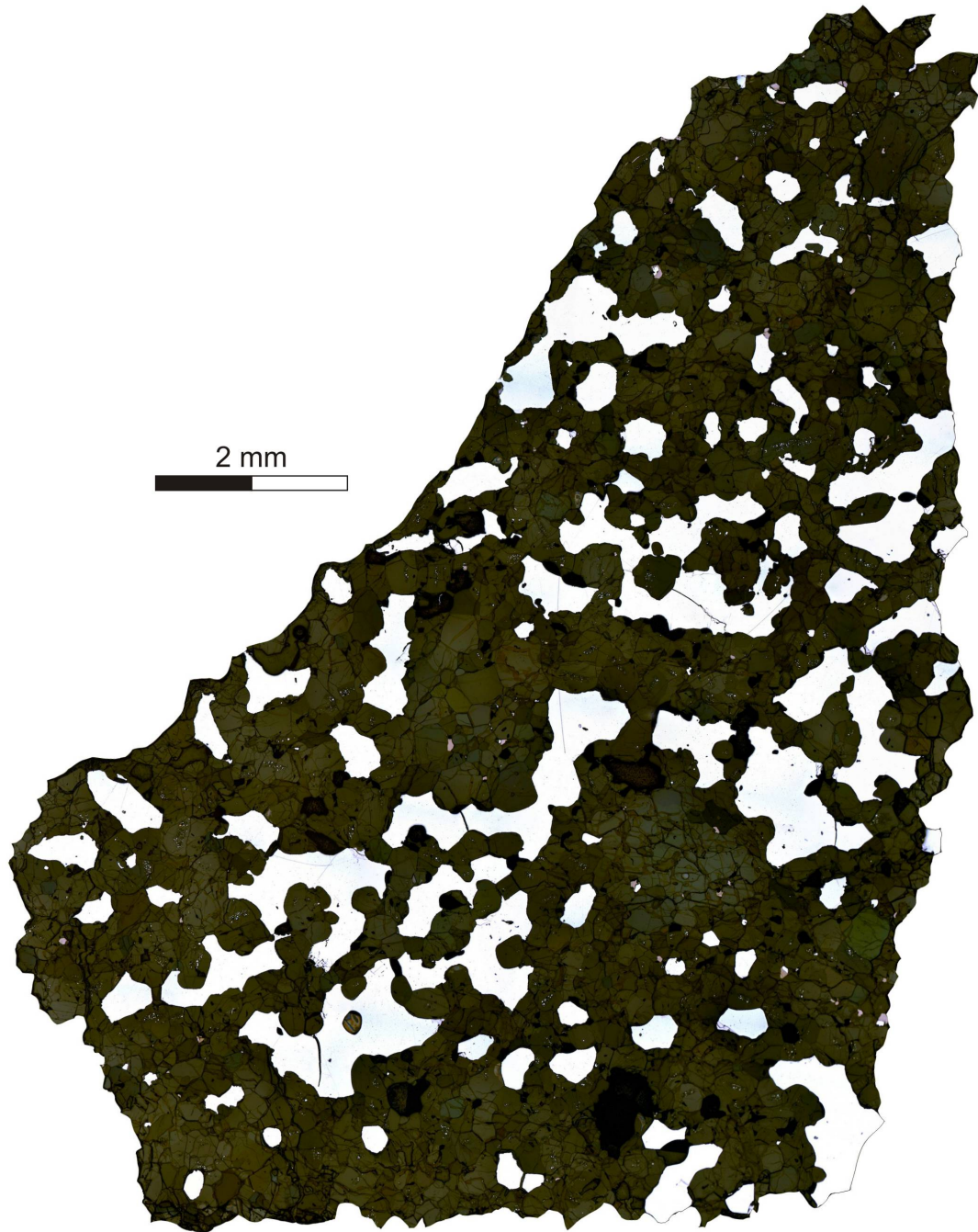
Figure 2.S2: Reflected light photomicrograph map of transitional meteorite EET 84302, 28 after Corder (2015). This meteorite serves as a particularly useful demonstration of the migration of metal in primitive meteorites – the FeNi metal in this sample appears to have “pooled” into large anhedral grains.
