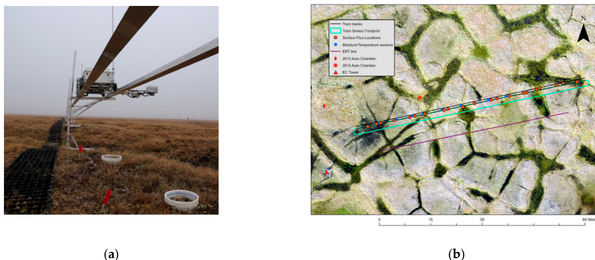
Figure 3. (a) Tram system installed at the Ngee-Arctic site, and (b) the aerial image of the tram track location with the point-measurement locations. In (a), the tram moves on two rails, carrying a sensor package on its arm. The flux chambers can be seen on the ground.
