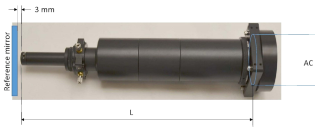
FIG. 1. The long distance aperture assembly that mounts to the tube of an ELCO-MAT 3000 autocollimator, with length L = 330 mm, equipped with adjustable circular apertures made of iris diaphragms. Note that the length is readily changed by removing sections of the extension tubing.
