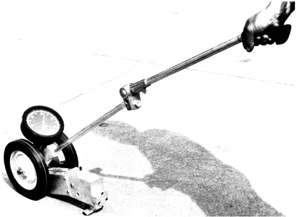
Figure 5: A Penn State Drag Tester. (5)
