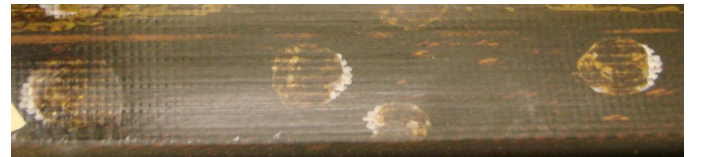
Fig.4. Several “bubbles” as they appear after a 1.9K test of TQS02a.
