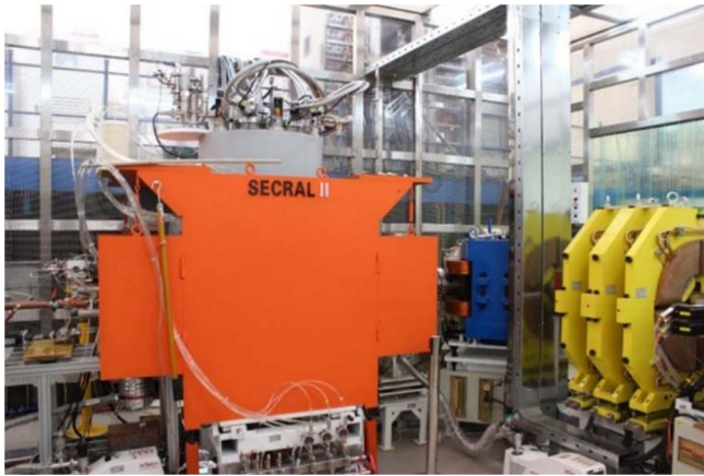
FIG. 32. The SECRAL-II ECR ion source at beam commissioning.
