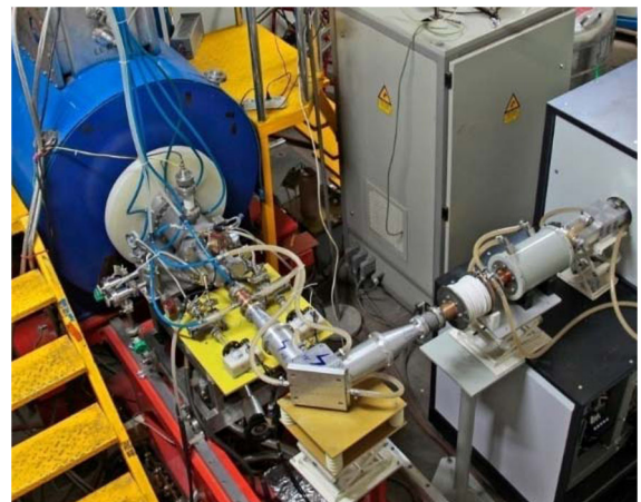
FIG. 4. The SECRAL source with 24 GHz microwave coupling.
