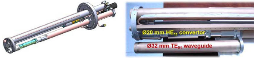
FIG. 16. Compact mode converter from TE_{01} to HE_{11} .
