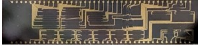
Figure 5.11: The picture of the fabricated silicon nitride chip with metal connections.
