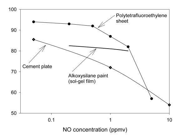
Figure 1. Fraction of NOx removed (%) for several samples containing TiO<sub>2</sub> nanoparticles, as a function of NO feed gas concentration (After Ibusuki, 2002). The fraction removed is nearly independent of NO concentration, but declines above 1ppm.
