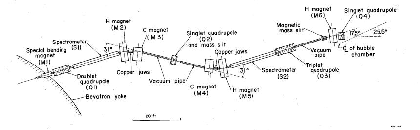
Fig. 1. Beam layout. The target (not shown) is the optical object for the first separation stage, which extends from the steering magnet M1 to the slit inside of quadrupole Q2. The first slit is the object for the second separation stage, which extends to the slit immediately in front of the magnet M6. The bubble chamber sees the image of the second slit.
