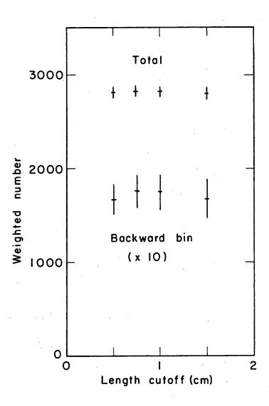
Fig. 6. For the data at 1.51 BeV/c, as a function of gap cutoff length, (a) the total weighted number of events, and (b) the weighted number in the backwardmost production angle bin. Since the  $K_1^0$  laboratory momenta are lowest there, this bin is most sensitive to the cutoff length. The data show that 0.5 cm is a sufficient cutoff length.
