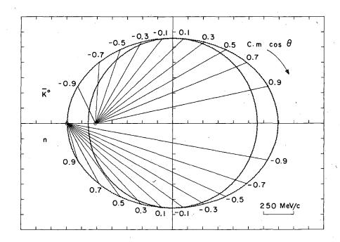
Fig. 4. An ellipse plot, displaying the kinematics of the reaction  $K^- + p \rightarrow \overline{K}^0 + n$  when the  $K^-$  laboratory momentum is 1.51 BeV/c. The radius of the circle equals the (final-state) c.m. momentum. Laboratory momenta and angles corresponding to various c.m. production  $\cos\theta$  can be read off directly;  $\overline{K}^0$  quantities are in the upper half, n quantities are in the lower.
