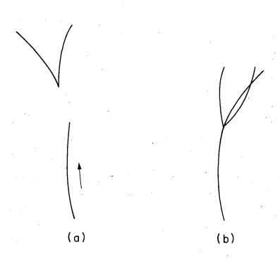
Fig. 3. Bubble-chamber topologies. (a) Charge-exchange scatter with subsequent  $K_1^0 \to \pi^+ + \pi^-$  decay of the  $\overline{K}^0$ ; (b)  $K^-$  decay into three charged particles.
