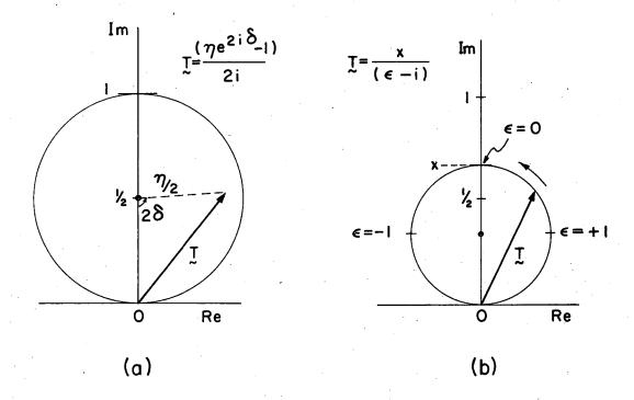
Fig. 18. (a) Unitarity bounds each (elastic) partial-wave amplitude within a circle of unit diameter. An amplitude  $\vec{T}$  is specified by two real numbers, conveniently  $\eta$  and  $\delta$ . (b) A resonance amplitude is parameterized with the Breit-Wigner form, which specifies its energy dependence; with increasing energy the amplitude traverses a circle of diameter x in the counterclockwise direction.
