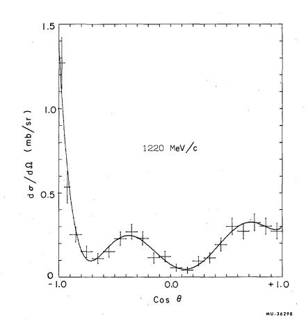
Fig. 11. Differential cross section for charge-exchange scattering at 1.22 BeV/c. The curve is taken from the fit with n = 6.
