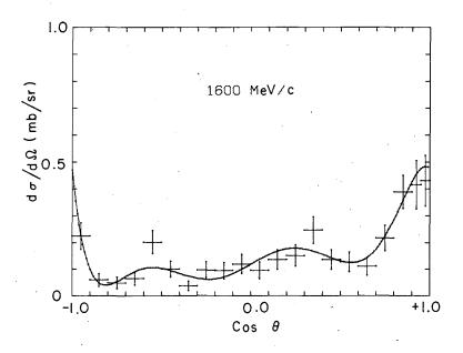
Fig. 14. Differential cross section for charge-exchange scattering at 1.60 BeV/c. The curve is taken from the fit with  $n_{max} = 7$ .
