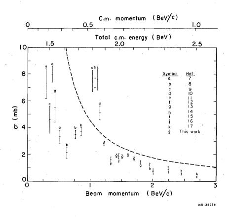
Fig. 10. The K-p charge-exchange cross section as a function of beam momentum, total c.m. energy, and c.m. momentum. The dashed curve is  $\pi \lambda^2$ .
