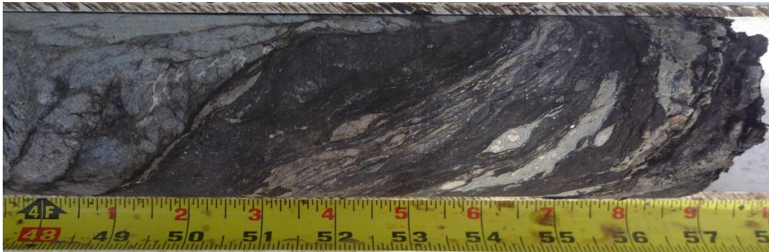
Figure 4-69. Foliated cataclasite at 91.74 m depth
