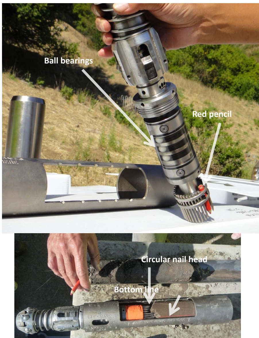
Figure 3-21. Core orientation tool. The probe attaches to the core retriever and is pushed against the top of the next core at the bottom of the hole together with the tip of the red pencil. Ball bearings lock to indicate the hole bottom direction. The shape of the circular nails is matched to that of core top. Red line on the core is drawn to mark the bottom direction of the hole.
