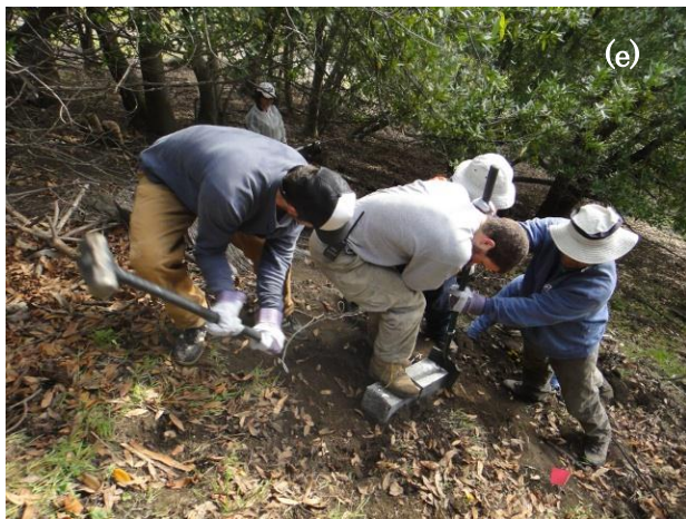
Figure 2-18: Seismic refraction survey photos: (a) P-wave geophone, (b) seismographic station, (c) seisguns, (d) seisgun blast, (e) S-wave source.
