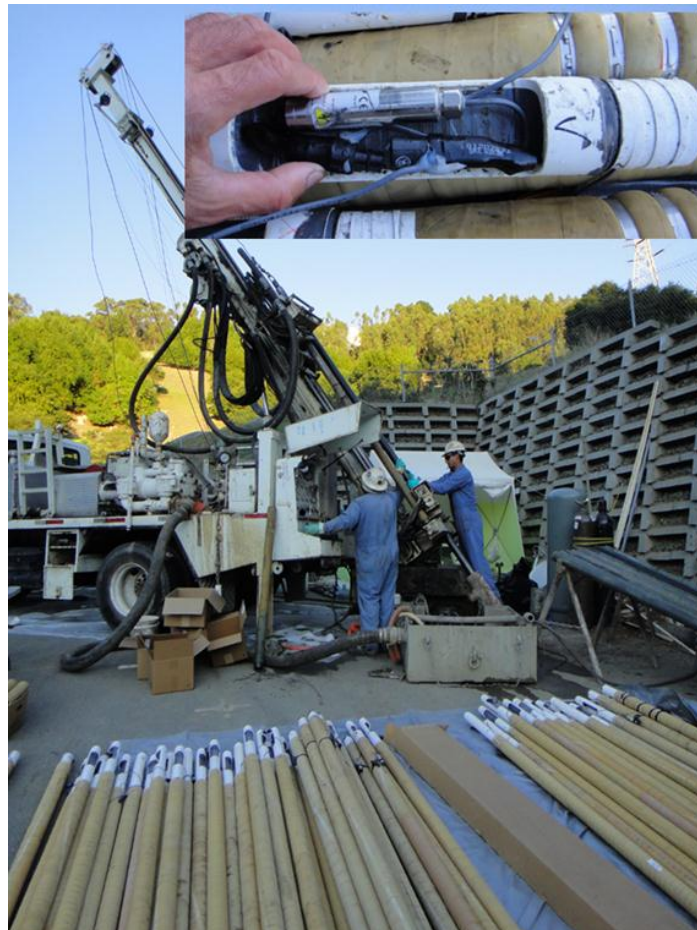
Figure 8-4. New concept packer system that continuously seal the borehole to avoid artificial short-cutting of pressure through the borehole. Their surfaces are made flush and neutrally bouyant in water.
