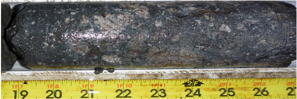
Figure 4-57. Dense material found in the contact between Orinda/San Pablo and Claremont.
