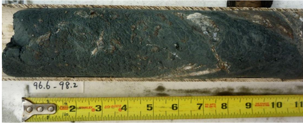
Figure 4-67. Deformation in the Orinda Formation in WF-3
