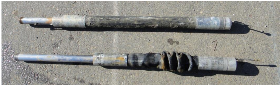
Figure 8-2. Damaged packer (below) and normal packer (above).
