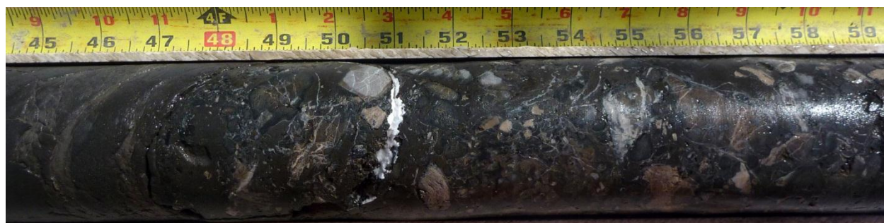
Figure 4-60. Conglomerate found in the contact between Orinda/San Pablo and Claremont.
