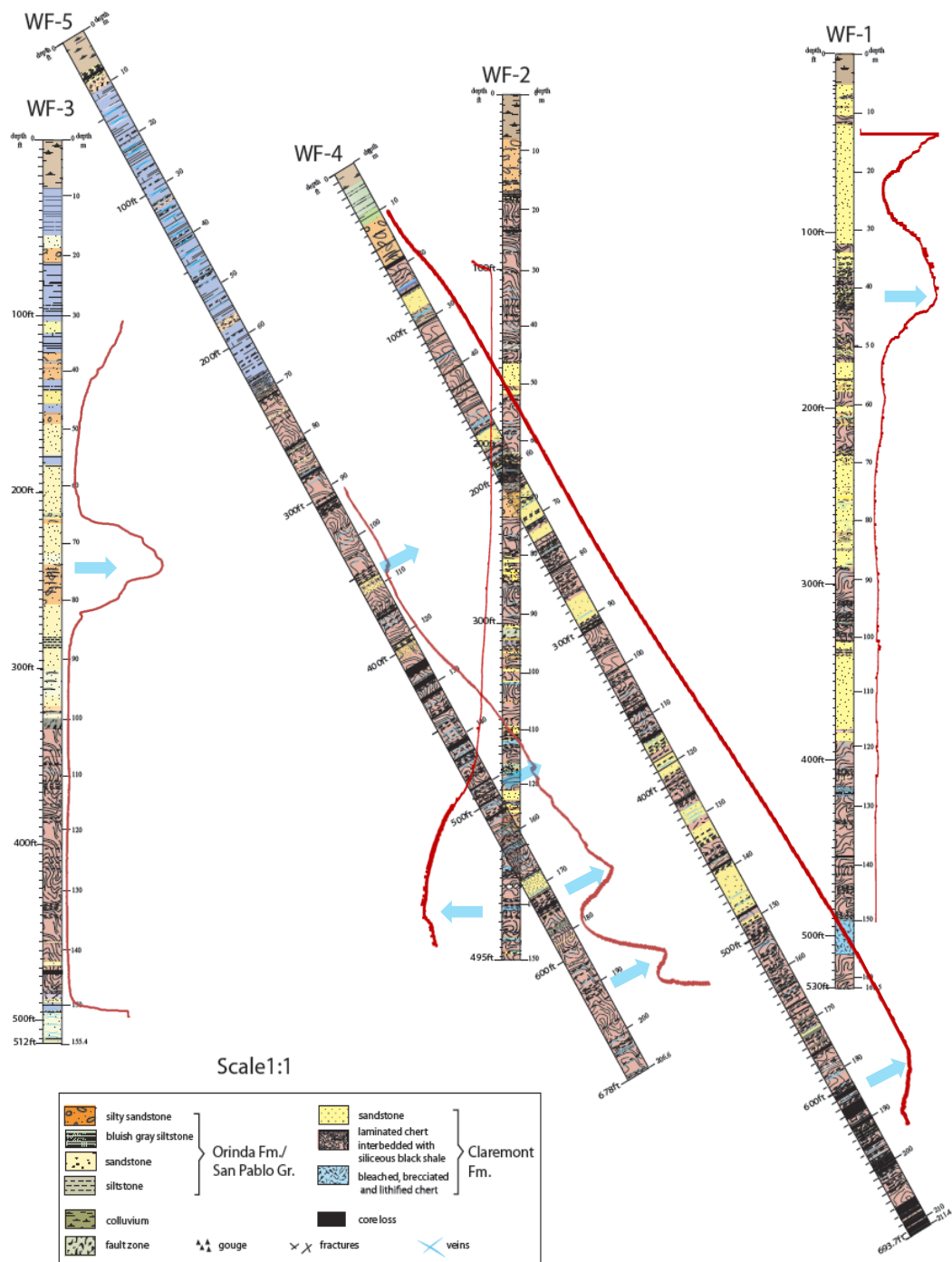
Figure 3-20. Flowing fluid electric conductivity log (FFEC) results (red lines) superimposed on the geologic columns of WF boreholes. Light blue arrows indicate inflow locations.
