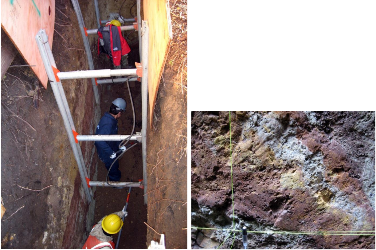
Figure 4-34. The typical mottled green sandy to siltstone and dark mudstone in TR2
