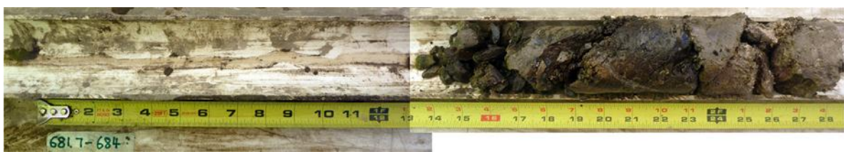
Figure 3-19. The BTV image from WF-4 at 681–684 ft (207.5 m–208.5 m). Also shown is the picture of the core from the same interval, most of which is not recovered. Note the very grainy image of the BTV, indicating that the rock is pulverized.
