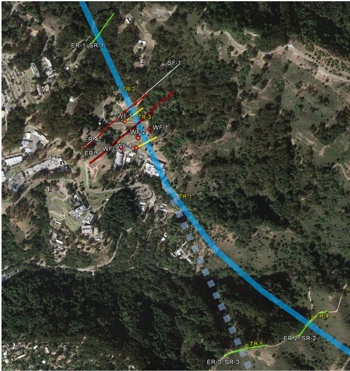
Figure 3-1. Sattelite picture showing the location of surface geophysical survey lines, trenches, boreholes and inferred traces of the Wildcat Fault (light blue solid and broken line).
