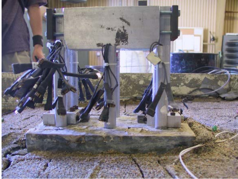
Figure 4. Side view of the pile cap, still embedded in the clay layer, after the surface layer of sand has been removed (Note the passive bulge on the uphill/right side).
