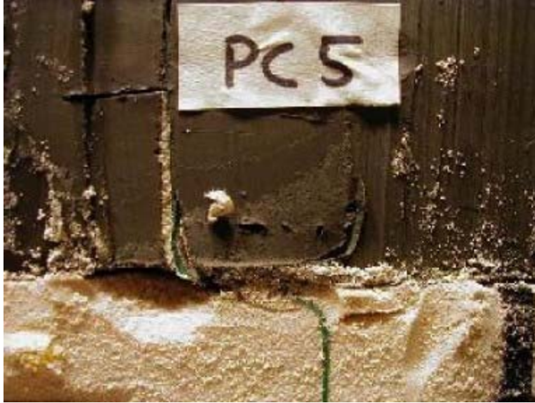
Figure 7. Side view of the contact between the liquefying loose sand layer and the overlying clay layer, with a vertical marker showing the discontinuity in deformation at the interface.
