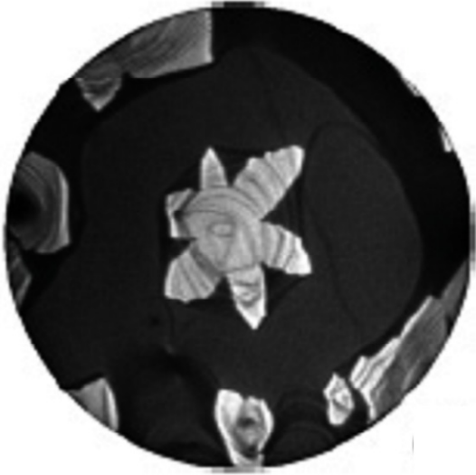
Figure 4.15 A graphene island on Cu(111) which nucleated where a screw dislocation intersected the substrate surface (FOV = 14.5 \mu\text{m} ).
