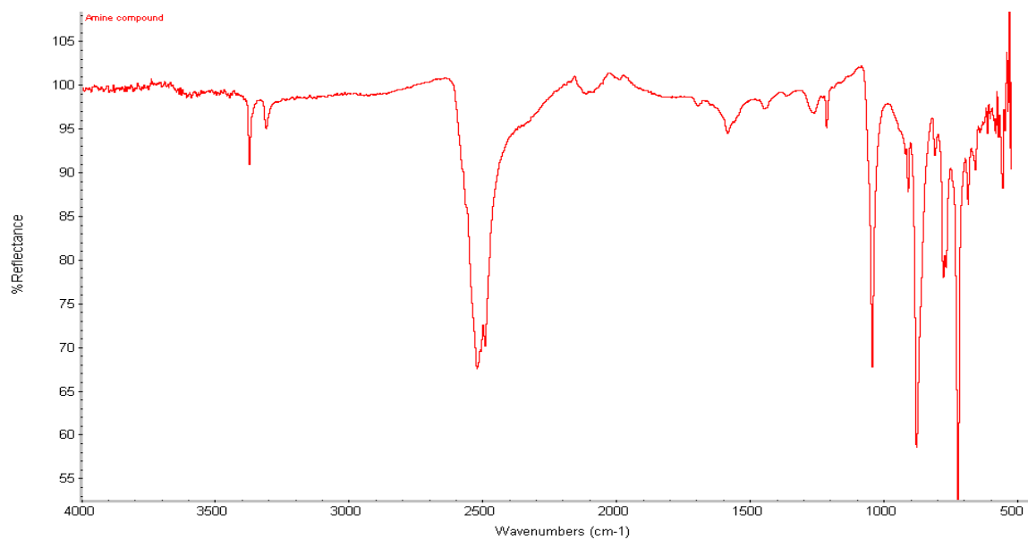
Figure 1-16. IR spectrum of 3\text{NH}_2[\text{Cs}^+] showing the B-H stretches near 2500\text{ cm}^{-1} .
