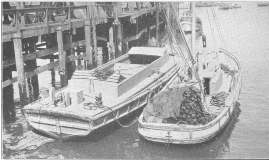
FIG. 2. A representative launch and lighter used for sardine fishing at Monterey. The lighter is towed by the launch on the fishing trips and the catch is loaded into it. This combination is known as a "lampara boat" in this paper, regardless of the type of net used. The above launch has a ring net piled on the stern. Photograph by J. B. Phillips, September, 1930.
