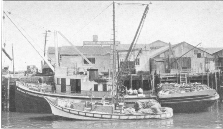
FIG. 3. A purse seine boat with a lampara launch alongside. The purse seine boat is slightly larger than the representative size used in the Monterey region for the past two seasons. The lampara launch is of representative size. The "lampara boat" fishing unit is not complete without the lighter (see Fig. 2). The lampara launches vary from 30–50 feet in length, and have engines ranging from 30–65 horsepower. The lighters that they tow are in the main from 40–50 feet in length. The purse seine boats vary in length from 55–85 feet, and have engines that range from 90–250 horsepower. (1929–1931.) Photograph by J. B. Phillips, October, 1930.
