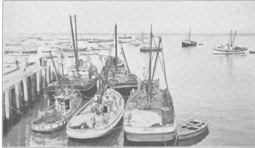
FIG. 1. Sardine fishing boats tied to Fishermen's Wharf at Monterey. These boats represent various types used in the Monterey region during the past two seasons. From left to right, the lower row: (1) A lampara launch that uses a ring net. This type of boat tows a lighter (see Fig. 2). Until 1930 this unit used a lampara net. (2) A new, large type of lampara launch that uses a ring net. This boat also tows a lighter. (3) A small purse seine type of boat using a ring net. The upper row shows two sizes of purse seine boats that use purse seines. The heavier construction of the purse seine makes it necessary to operate the net with the aid of a turntable. Photograph by J. B. Phillips, September, 1930.
