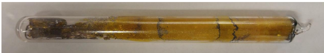
Figure S4. Vapor Transport tube after the transport experiment shows the transported \text{PbI}_2 on the right side of the image. The black solid on the left hand side is the remaining \text{AuPb}_2\text{I}_7 grown on \text{PbI}_2 , with a dominant amount of metallic gold. This was in the hot zone.
