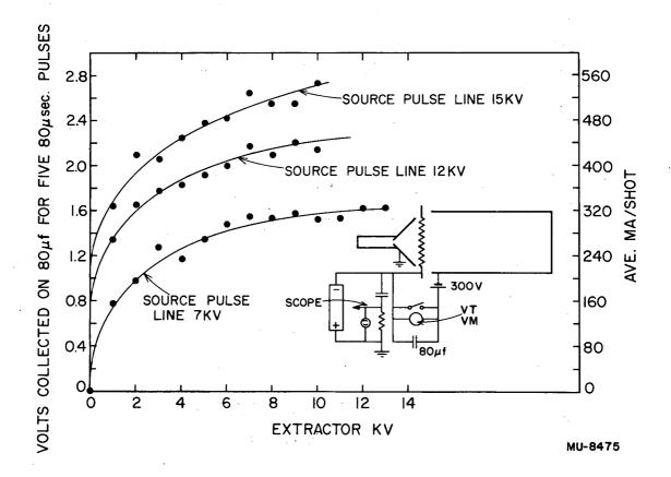
Fig. 5. Ion current versus extractor voltage for grid-type axial extraction.
