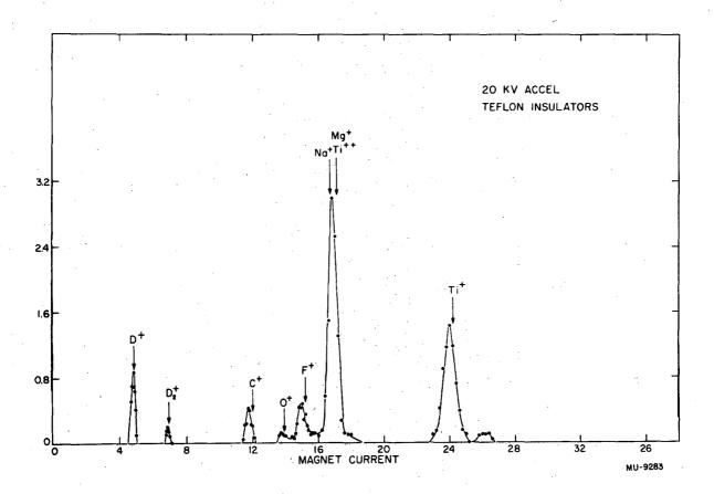
Fig. 12. Mass spectrum for Ti-D with teflon insulators.
