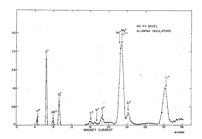
Fig. 11. Mass spectrum for Ti-D with alumina insulators.
