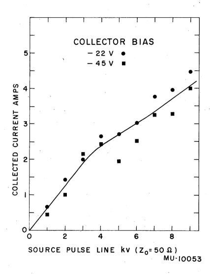
Fig. 2. Ion current versus charging voltage for filament-type source.
