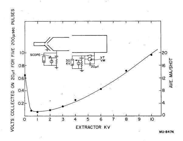
Fig. 4. Ion current versus extractor voltage for aperture-type axial extraction.
