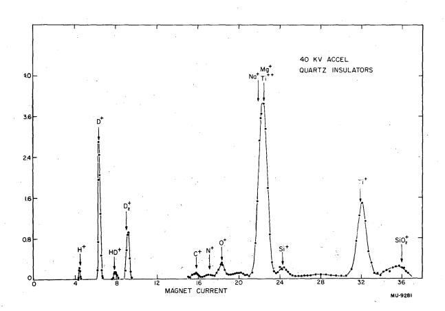
Fig. 10, Mass spectrum for Ti-D with quartz insulators.
