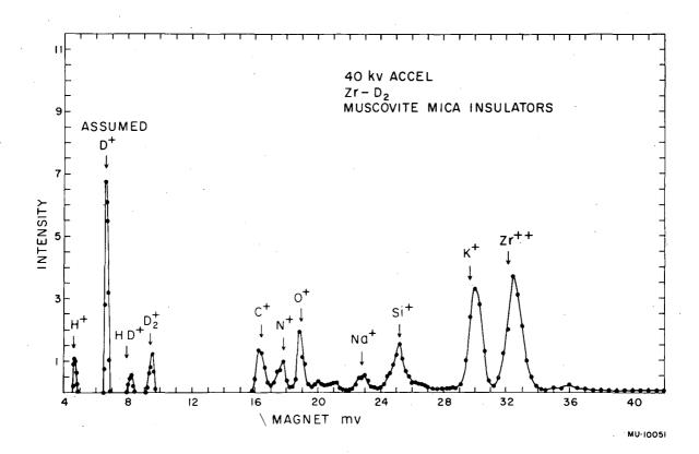
Fig. 13. Mass spectrum for Zr-D with mica insulators.
