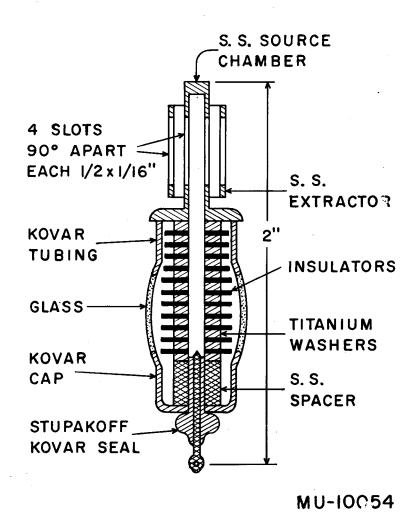
Fig. 6. Confined-volume source with exit geometry for radial extraction.
