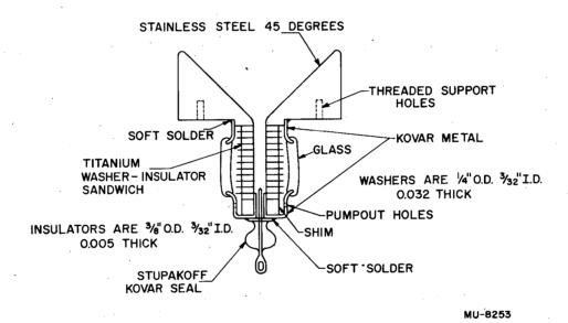
Fig. 3. Confined-volume source with exit geometry for axial extraction.
