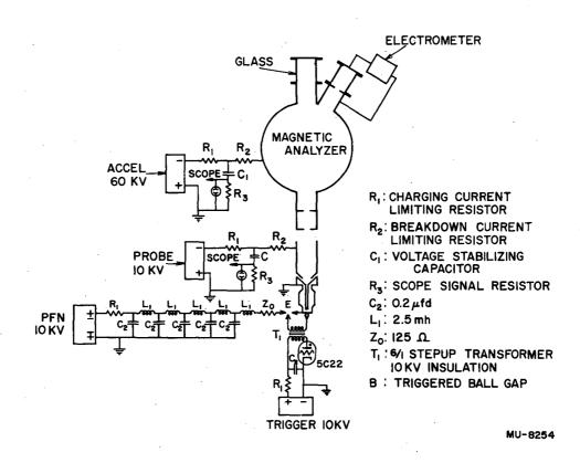
Fig. 8. Magnetic mass-analysis system and associated electronics.
