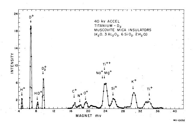
Fig. 9 Mass spectrum for Ti-D with mica insulators.
