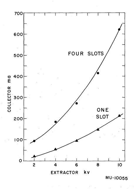
Fig. 7. Ion current versus extractor voltage for radial extraction.
