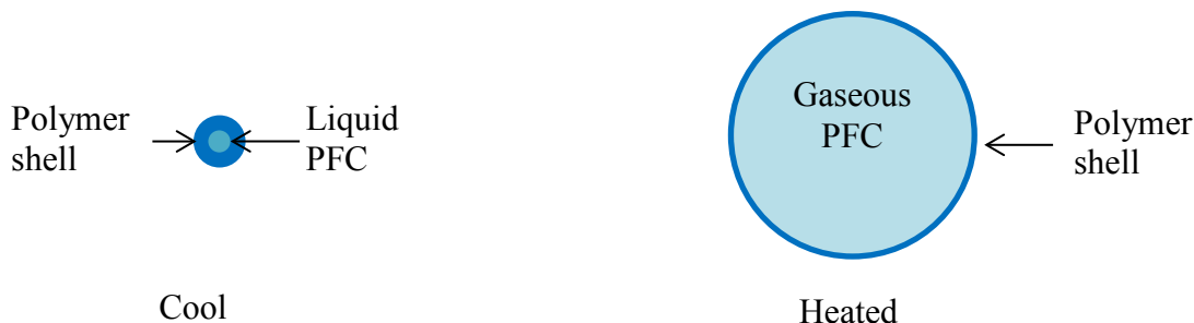
Figure B.1 The volatile cores of the microcapsules investigated herein vaporize upon heating.
