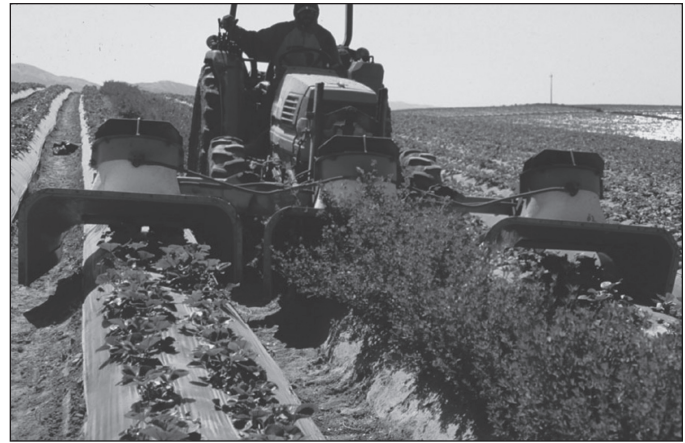
An employee at Pacific Gold Farms uses a tractor-mounted bug vac to vacuum an alfalfa trap crop.
