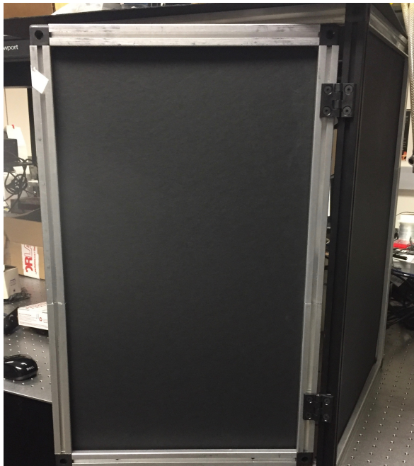
Figure 14: A light-tight enclosure system built to eliminate ambient light contamination.
