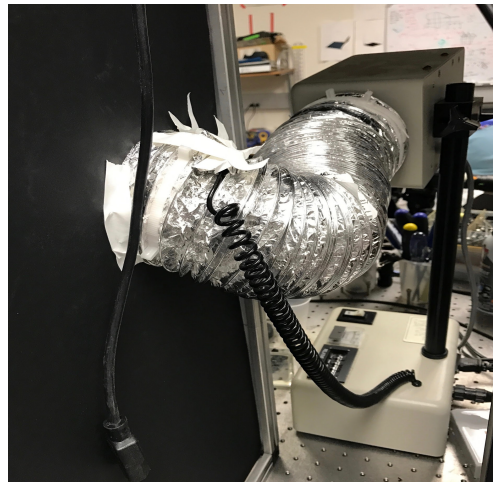
Figure 13: An air stream incubator (ASI 400m Nevtek, Williamsville, VA) integrated to our imaging setup to maintain a suitable body temperature for the subject under study. The heat was directed toward the subject via a flexible aluminum pipe
