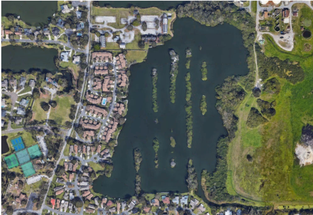
Figure 2. Lake Somerset and its islands. A dragline operator mines phosphate in strips, much like Americans mow a lawn. The dragline mines a row, removing the top layer of overburden to one side, pivots, and begins mining a new row parallel to the last.
