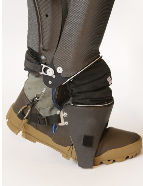
Figure 4.25: The Otherlab exoskeleton utilizes cloth pneumatic actuators for toeoff. This novel cloth actuator functions equivalently to a pneumatic expansion cylinder, but with much lower added weight.
