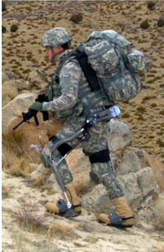
Figure 1.5: HULC (Human Universal Load Carrier) was developed with load carriage in mind, but the device is metabolically detrimental during running.
