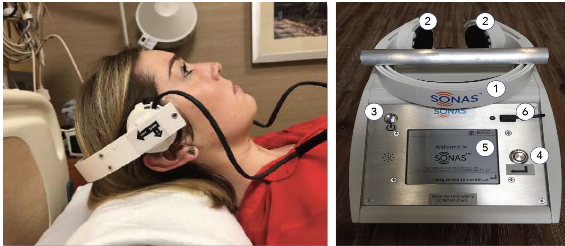
Fig. 1 Left: SONAS ® headset. Right: SONAS ® device, pre-commercial/trial version. Positioning of the transducers above the temporal bone window on both sides of the head with subject in supine position. 1: headset, 2: transducer, 3: power button, 4: "enter" button, 5: LCD screen, 6: USB port. Size: 19 × 19 × 12 cm. Weight: 2,2 kg
