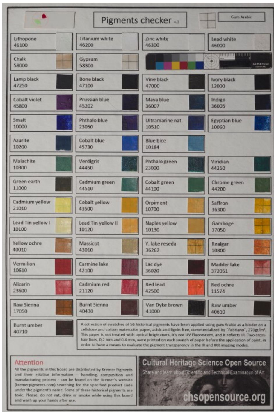
Figure 2.11. The Pigments Checker developed by Cultural Heritage Science Open Source (visible light).
