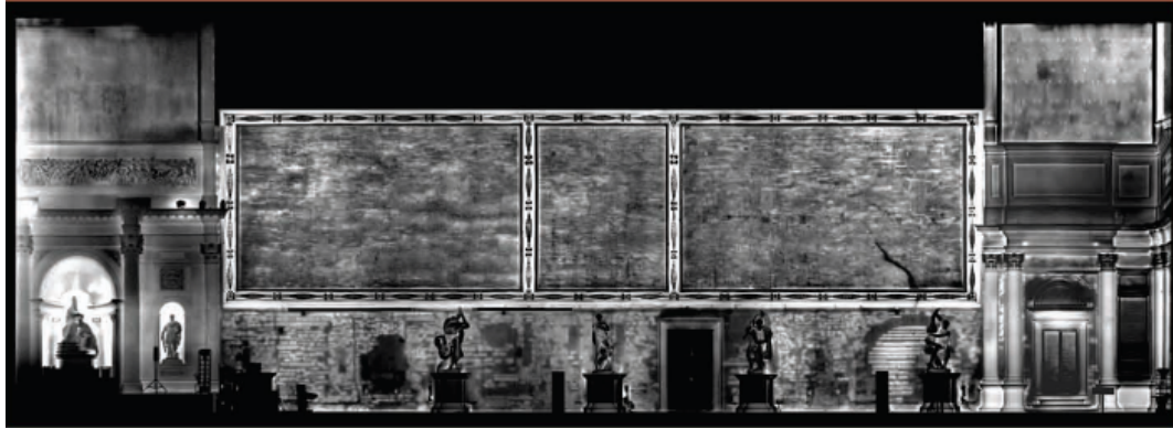
Figure 4.11. Thermogram of the East Wall of the Hall of the 500
