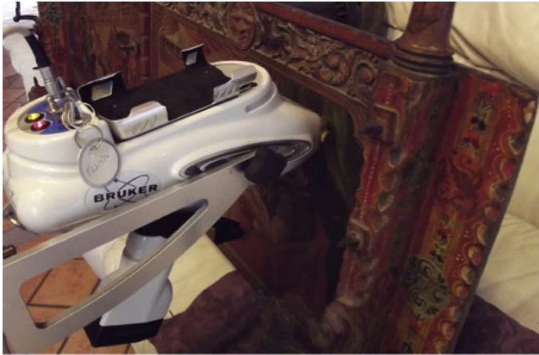
Figure 5.8. Portable XRF instrument supported by a tripod, shown here scanning one point on the Sicilian Cart.
