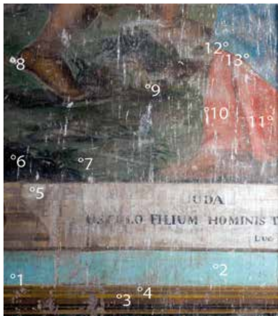
Figure 4.27. Areas analyzed by pXRF and FORS on The Kiss of Judas mural painting.
