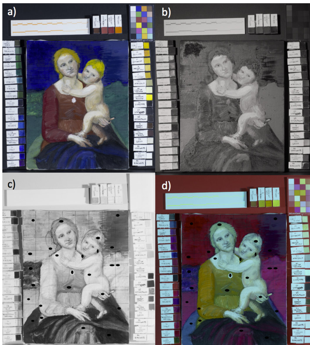
Figure 6.3. Technical Photography of the Pratt Madonna surrounded by pigment swatches: a) VIS, b) UVR, c) IR, d) IRFC.
