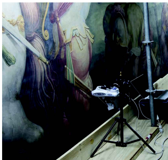
Figure 4.18. XRF point analysis using the Bruker Tracer III/SD mounted on a tripod.
