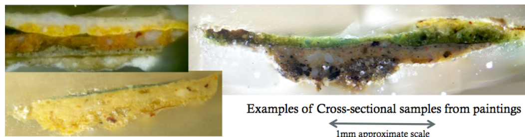
Figure 2.8. Three examples of cross-sectional paint samples, showing the variability in layering and grain size. [1]
