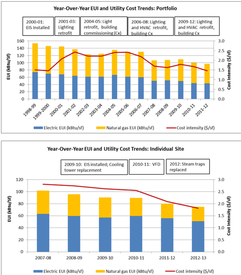
Figure 1. Year-over-year energy use and utility cost trends for a portfolio (top) and single building (bottom), with annotations to indicate major projects and year of EIS installation
