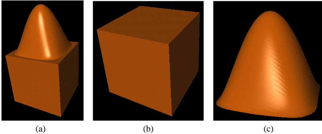
FIGURE 2: A trivariate solid: The complete solid is shown in (a); The boundary face patches are shown in (b); and the implicit boundary surface is shown in (c).
