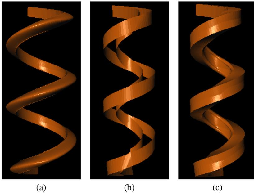
FIGURE 3: Image (a) shows the implicit boundary surface swept along the helical path. Image (b) is the locus of characteristic curves of the boundary face patches along the path. Image (c) shows the swept edges of the image boundary patches. The resulting envelope is the union of these surfaces.
