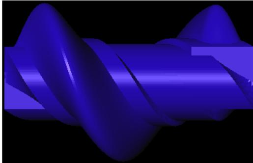
FIGURE 7: Image is the swept surface of the trivariate solid rotating a total of  $360^\circ$  along a horizontal path.
