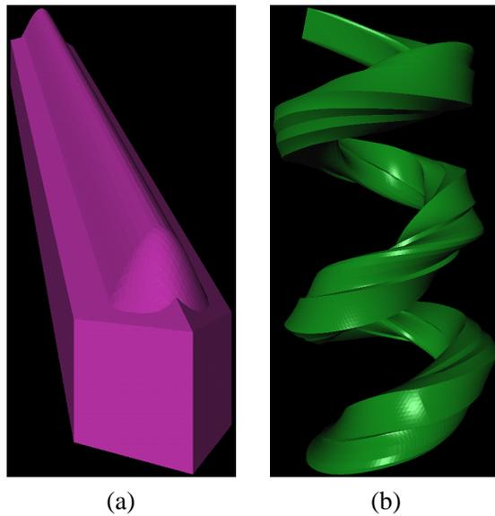
FIGURE 4: Image (a) is the swept surface of the trivariate solid from Figure 2.1 along a diagonal. This is an example of an upright sweep. In image (b), the same trivariate solid is swept along the helix from Figure 3, except in a rotating sweep. The total amount of rotation is  $360^\circ$ .
