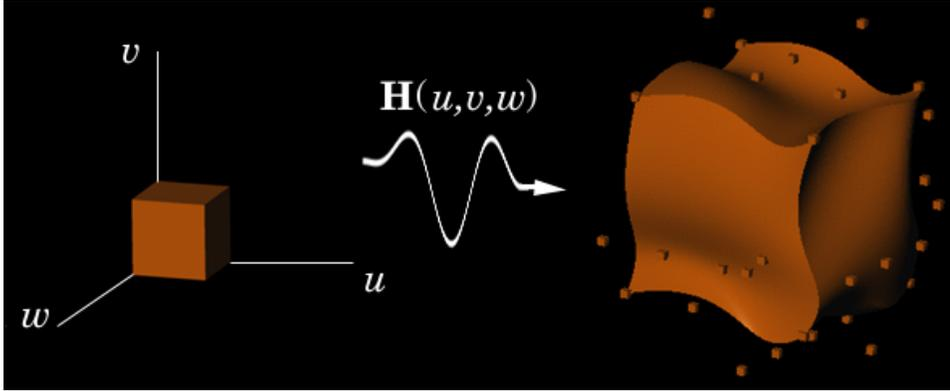
FIGURE 1: A trivariate tensor-product Bézier Solid  $\mathbf{H}(u, v, w)$  shown with 64 control points (most of which are inside the solid).
