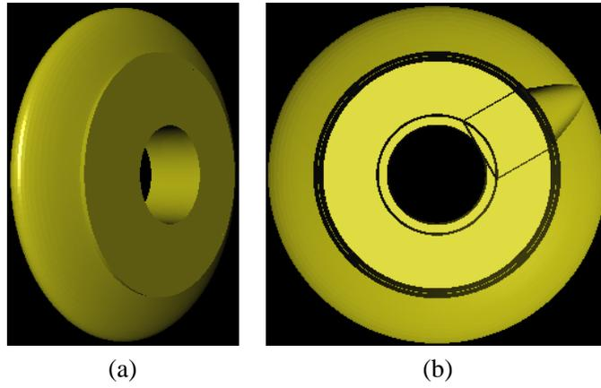
FIGURE 5: Image (a) shows the local sweep of the trivariate solid swept along a plane circle. Image (b) is a clipped version of image (a). The generator is seen here in its starting (and finishing) position.
