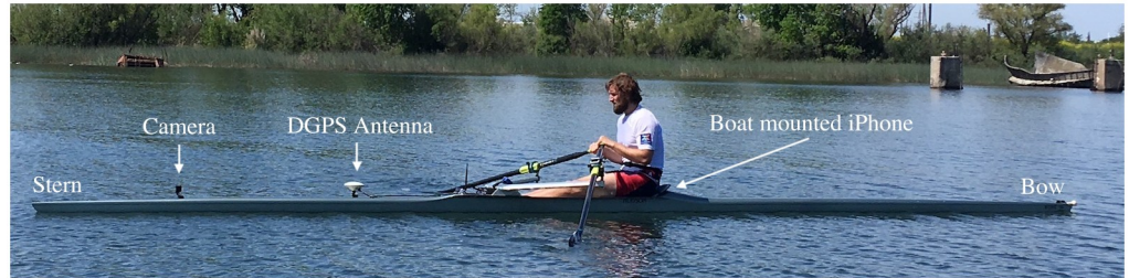
Fig 8. Sensor locations during elite trials. 2004 Hudson heavy-weight with the elite rower, annotated for experimental hardware. Note the DGPS antenna is clearly visible to the sky (above 15 degrees from horizontal in all directions it is with a clear view to the sky). The individual pictured has given written informed consent (as outlined in PLOS consent form) to publish these case details.
