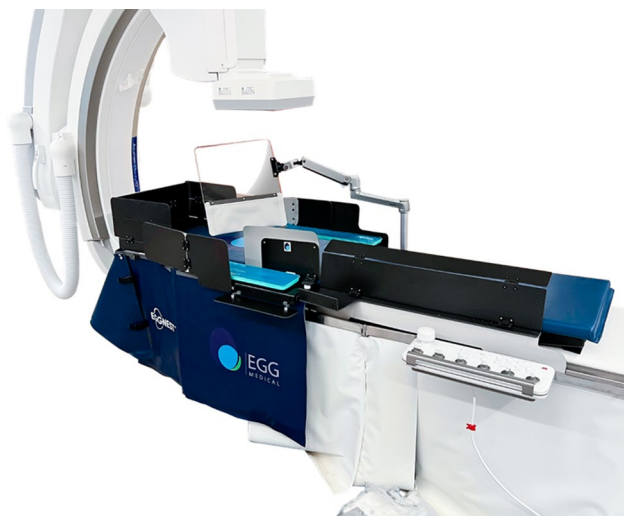
Fig. 1 The EggNest XR system is comprised of a carbon-fiber sled base and mattress, with built in CPR board, as well as shields positioned between the operator and patient to mitigate scatter radiation exposure with 0.5 mm lead-equivalent. (Reprinted with permission from EggNest XR Medical)
