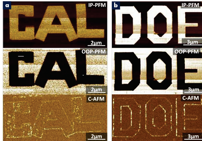
Figure 4.7: “CAL” and “DOE” switched pattern showing conduction at written domain walls. (a), (b) From top to bottom are IP-PFM, OOP-PFM, and C-AFM images of the switched area, respectively
