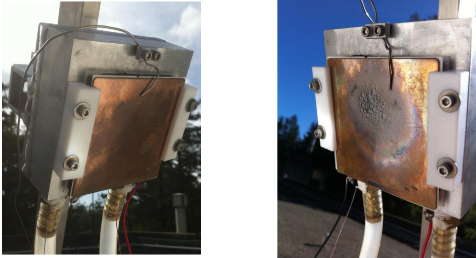
Figure 4.3: Pictures of the first generation solar receiver before and after heating. Right image shows the localized damage caused by the intensely concentrated solar irradiation on the copper heat spreader.
