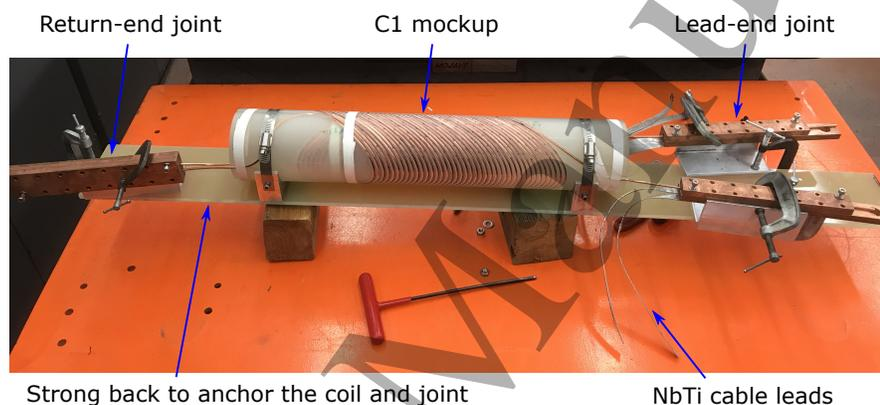
**Figure 4.** A 1:1 mockup model for C1. The model was used to develop and verify the assembly concept and to determine and confirm the required conductor length as provided by the CAD model. The winding of Layer 1 (inner layer) can be seen through the mandrel of Layer 2.
