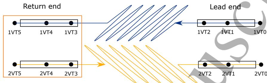
**Figure 5.** The voltage taps installed on each layer of C1. Black boxes are terminations. Current flows from Layer 1 to Layer 2 as indicated by the arrows. A praying-hand joint (orange box) connected both layers at the return end.
