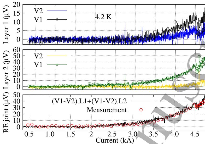
**Figure 12.** The voltage across each layer and the return-end joint as a function of current at 4.2 K. The linear resistive component was removed. The voltage inside the terminations from both layers added to the measured superconducting to normal transition in the return-end joint.
