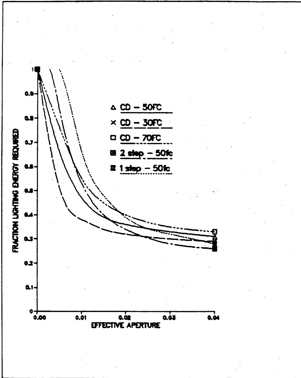
Figure 2. Lighting energy requirements with daylighting for skylight module in Los Angeles; comparison of lighting level and control.
