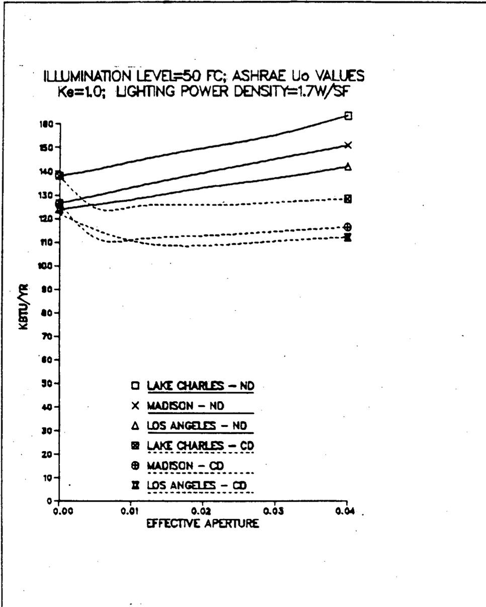
Figure 6. Peak electrical demand for skylight modules. Shows continuous dimming vs. no daylighting controls.
