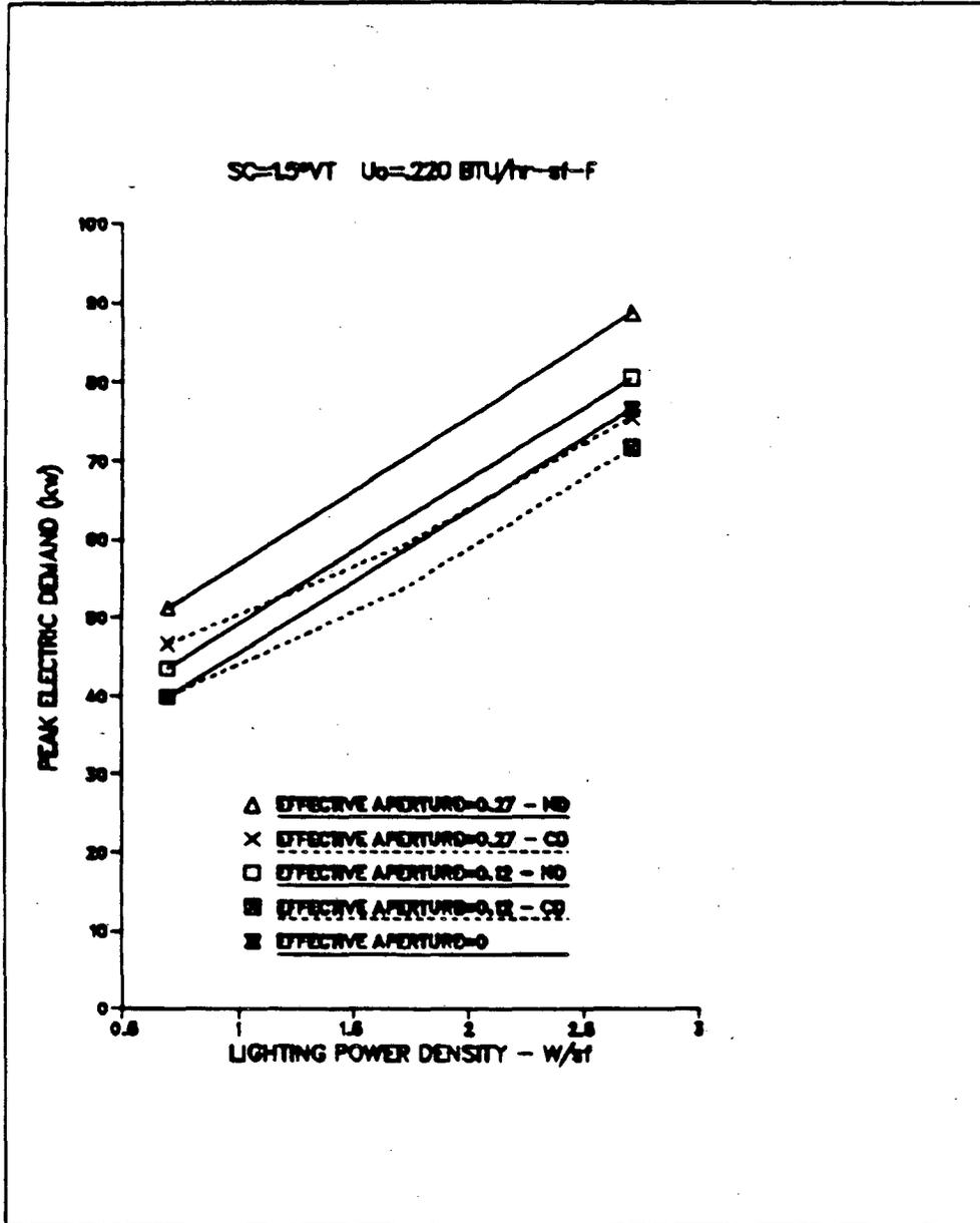
Figure 5. Peak electrical demand as a function of lighting power density: Los Angeles, office module with windows; continuous dimming vs. no day-lighting controls.
