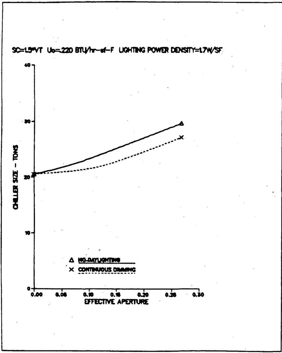
Figure 4. Chiller size as a function of effective aperture for office module with windows; continuous dimming vs. no daylighting controls.
