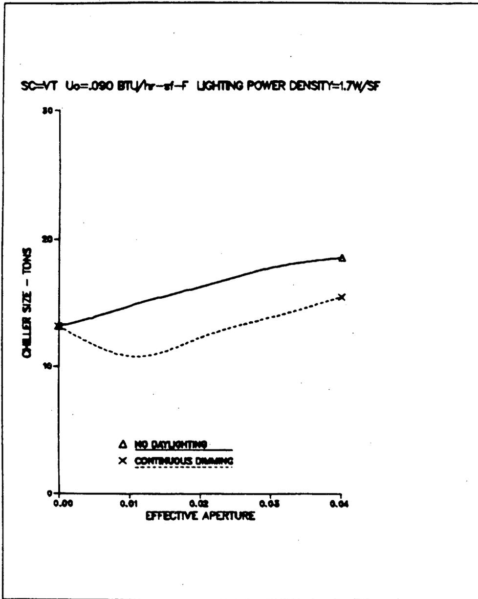
Figure 9. Chiller size as a function of effective aperture for skylight module in Los Angeles. Shows continuous dimming vs. no daylighting controls.
