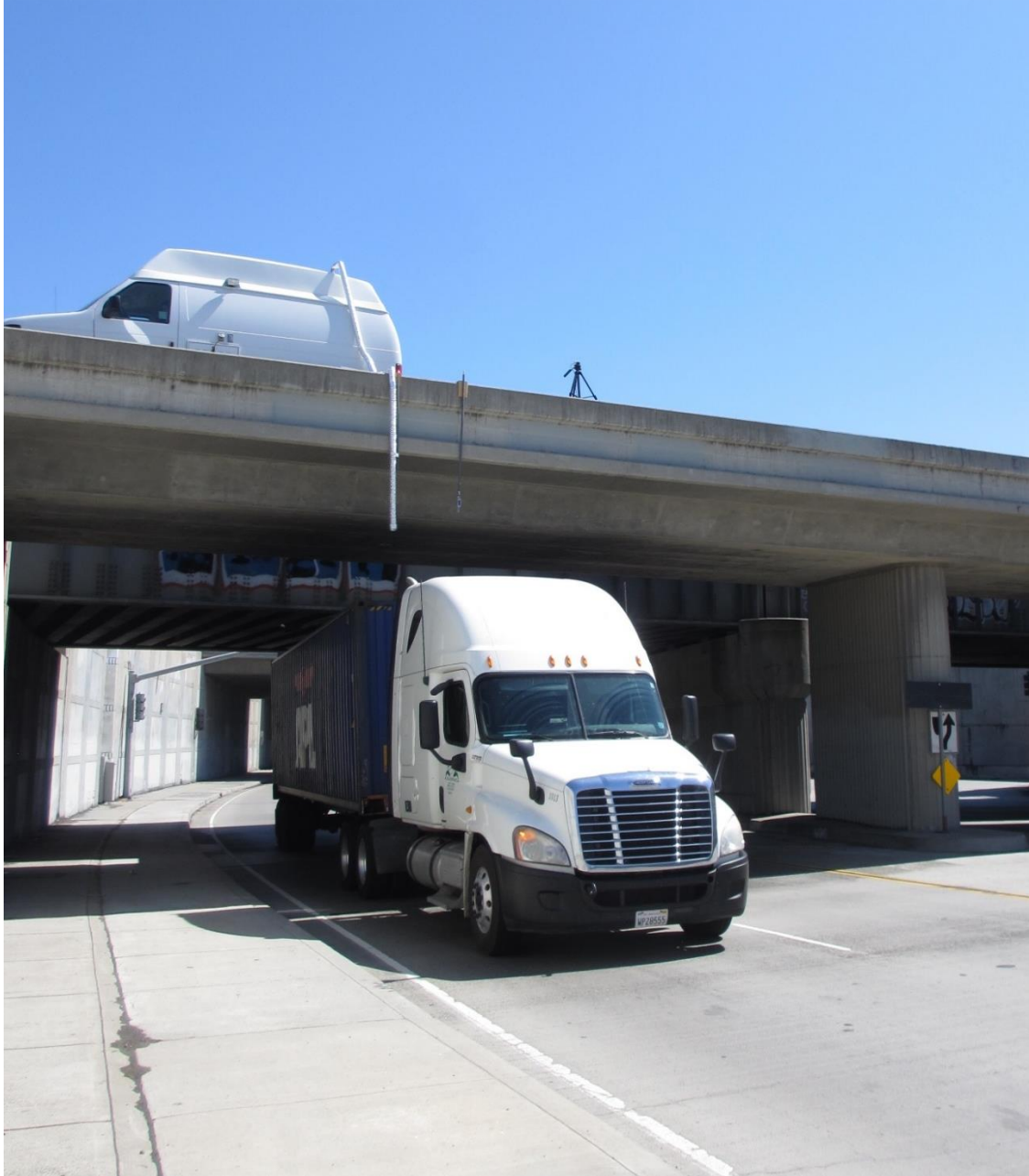
Figure 2.2 Instrumented van positioned on an overpass sampling the exhaust from a truck en route to the Port of Oakland.
