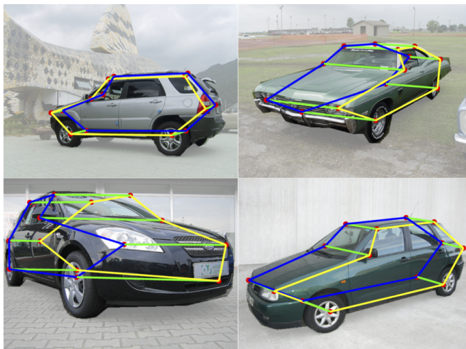
Figure 2.4: NRSfM camera estimation: Estimated cameras visualized using a 3D car wireframe.
