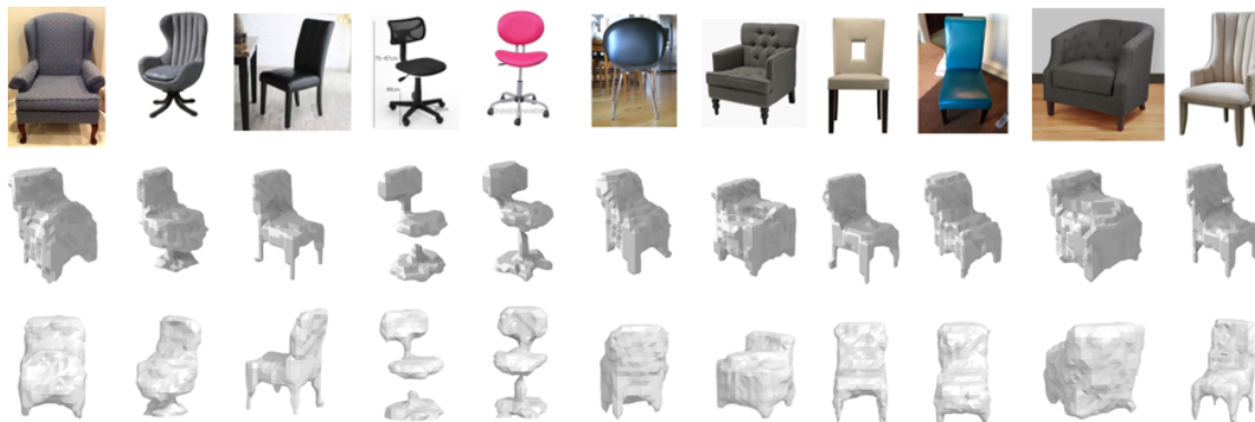
Figure 3.10: Visualization of predictions using the Stanford Online Product Dataset. (Top) Input image. (Middle) Predicted shape in the emergent canonical pose. (Bottom) Predicted shape rotated according to the predicted pose.
